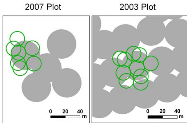
Figure 4. Spatial relationship between LVIS footprint (open circles) and plot range (solid circles). Plot level LVIS products were obtained by averaging LVIS data for footprint centers located within a 5 m radius circular centered at each plot center.
