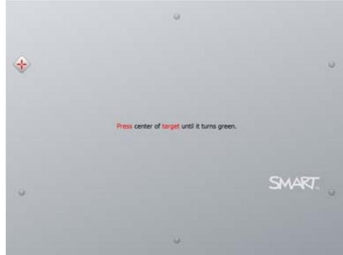
5. Use the tip of a pen tray pen to press the red targets as they appear. Move the tip to the center of each target until the target turns green, and then lift the pen. When you remove the pen, the target moves to the next calibration point.
