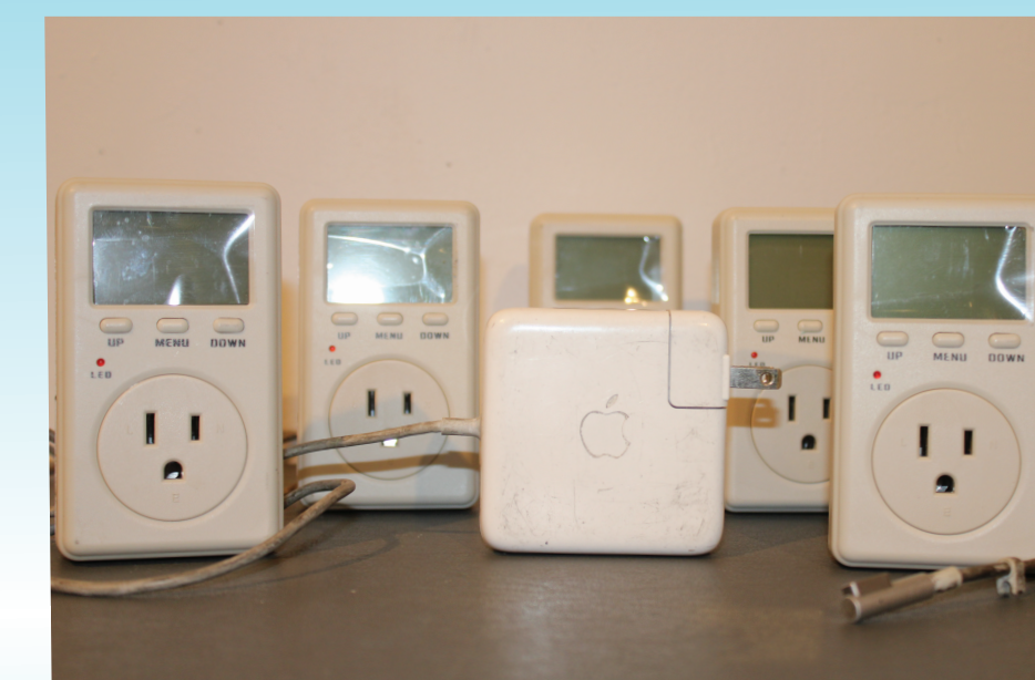
All six ammeters used in the experiments were the Multifunctional Mini-ammeter model number DO2A made by Shenzhen Wanfang Hi-tec co.
