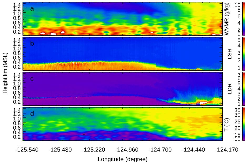
**Figure 8-16.** (a) WVMR, (b) LSR, (c) LDR and (d) temperature cross-sections along 40° N from the ocean (left side) to the coast around the Shelter Cove on June 30, 2016, based on MARLi measurements from the UWKA. Water vapor mixing ratio (WVMR), Lidar scattering ratio (LSR), Lidar depolarization ratio (LDR) (Wang, personal communication).
