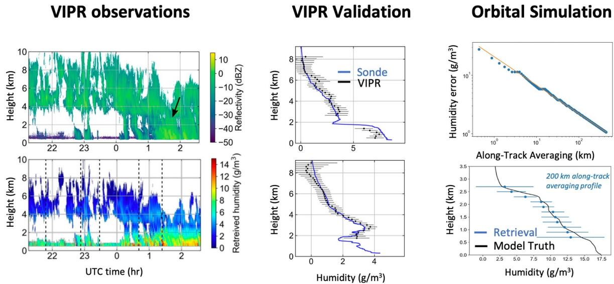
**Figure 8-11.** An example of a cloud and water vapor curtain from the Vapor In-Cloud Profiling Radar (VIPR; left), example validation of VIPR water vapor retrievals (middle), and results of a simulation of DAR retrieval performance from an orbital platform observing shallow precipitating marine cumulus (Roy, personal communication).
