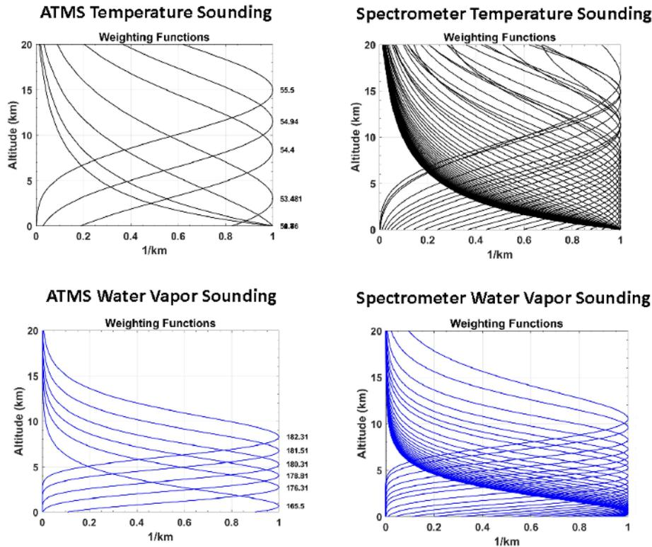
**Figure 8-14.** (Left) Weighting functions for the ATMS temperature (top) and water vapor (bottom) sounding channels. (Right) Example weighting functions for a hyperspectral MW sounder (Brown, personal communication).
