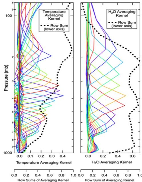
**Figure 8-12.** Sample of AIRS single foot-print averaging kernels, row sums of the averaging kernels and approximate vertical resolutions for temperature (left) and water vapor (right). From Irion et al. (2018).
