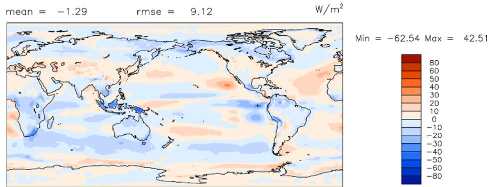
**Figure 4-4.** Differences in TOA shortwave (SW) cloud forcing ( $\text{Wm}^{-2}$ ), annual long-term mean, between the latest NCAR atmospheric model (CAM6) and the CERES observations. From Neale et al. (2021).
