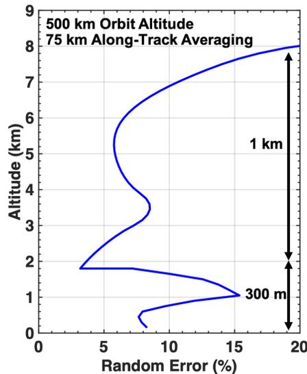
**Figure 8-10.** DIAL random error simulations from an orbital platform observing a mid-latitude clear air scene. Different vertical averaging in the PBL and free troposphere aloft allow for optimization of the retrieval precision (random error) (Nehir, personal communication).
