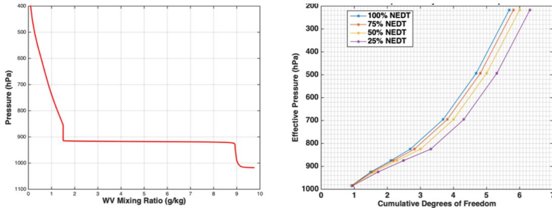
**Figure 8-13.** (Left) Simulated water vapor profile for a well-mixed PBL over the subtropical ocean from a Large-Eddy Simulation (LES). (Right) cumulative degrees of freedom from IASI with different levels of noise (Wilson, personal communication).
