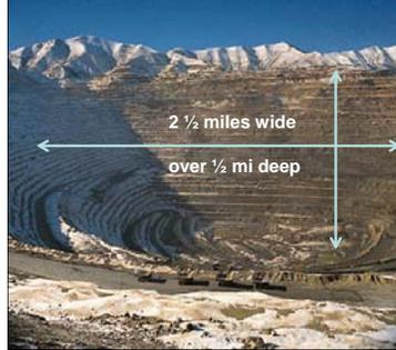
Open pit mining is a means of extracting minerals from the earth by digging a bowl-like pit that gets wider and deeper with use.
